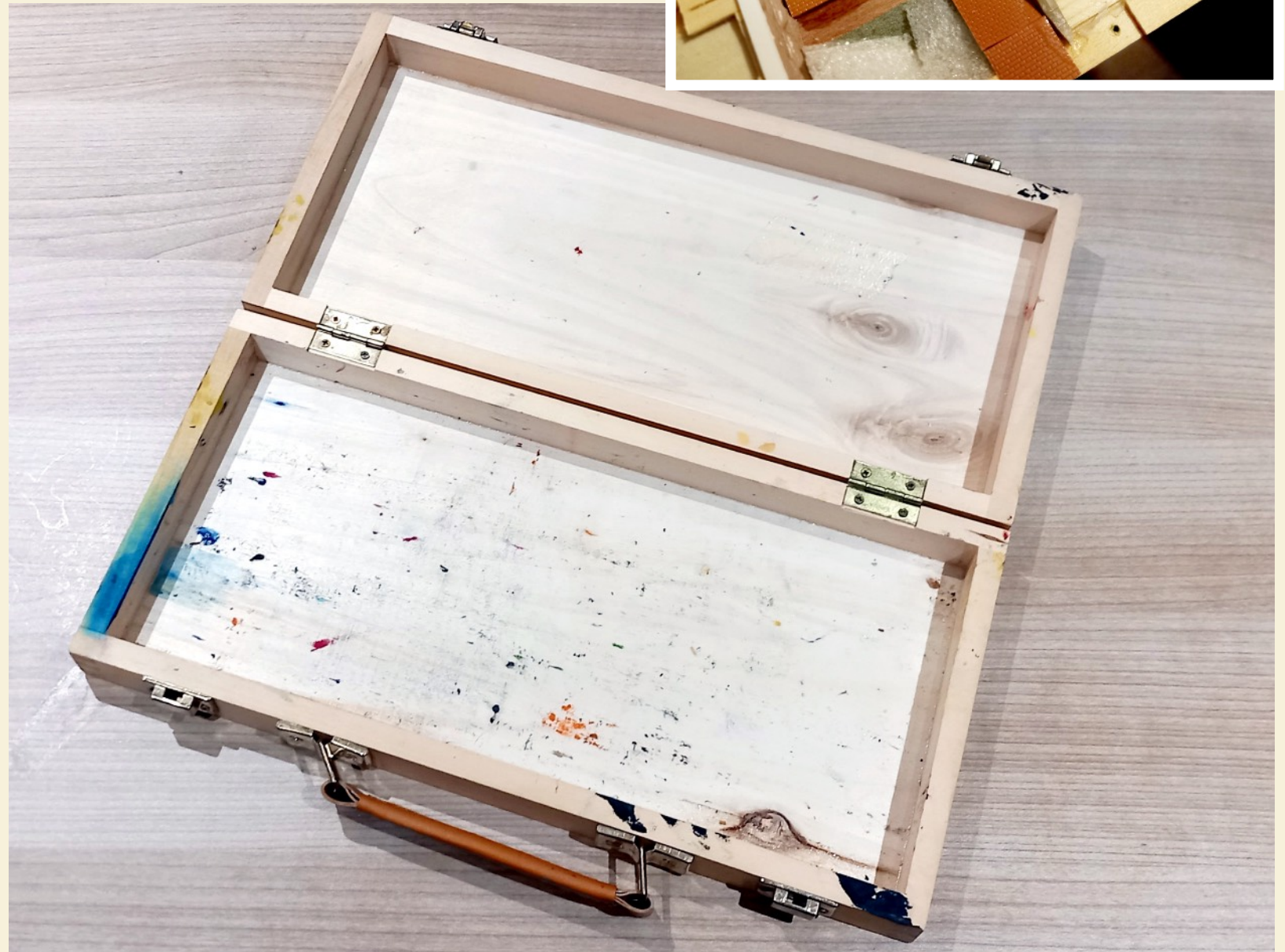
The storage box that started the project. In the inset picture you can see how the hinges were relocated in order to have the box close correctly
