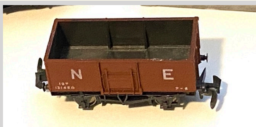
The modified Rapido coupling
